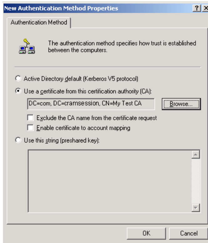
Figure 13 – The New Authentication Method Properties Dialog Box Enables You to Configure IPSec Authentication Methods
