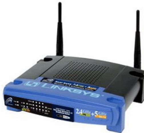
Figure 47: A wireless access point (AP)
