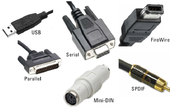
Figure 5: I/O port form factors
