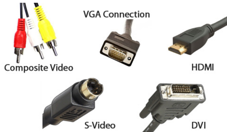
Figure 4: Video connector form factors
