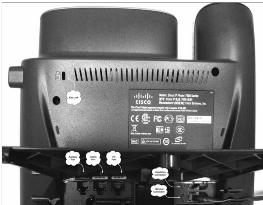
Figure 6-2: Cisco IP phone ports.
