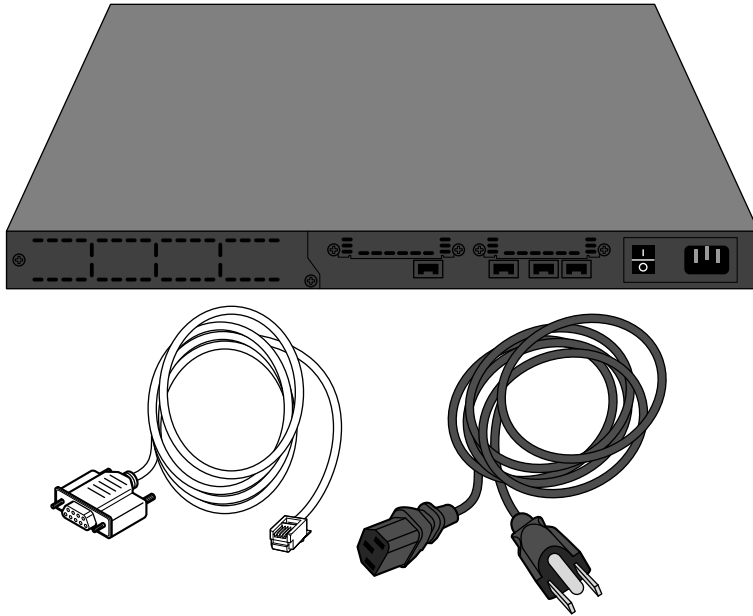
Figure 2-2: Cisco 2621 router and accessory items — Rear panel.
