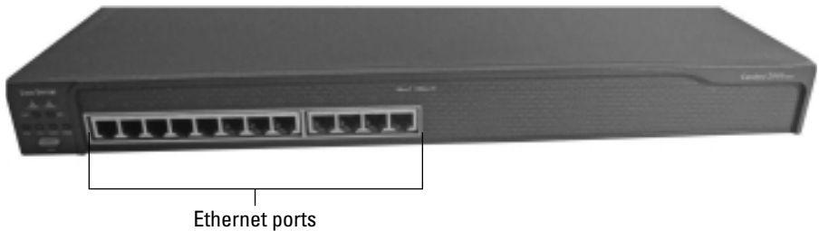
Figure 1-11: Fast Ethernet ports on a Cisco switch.
