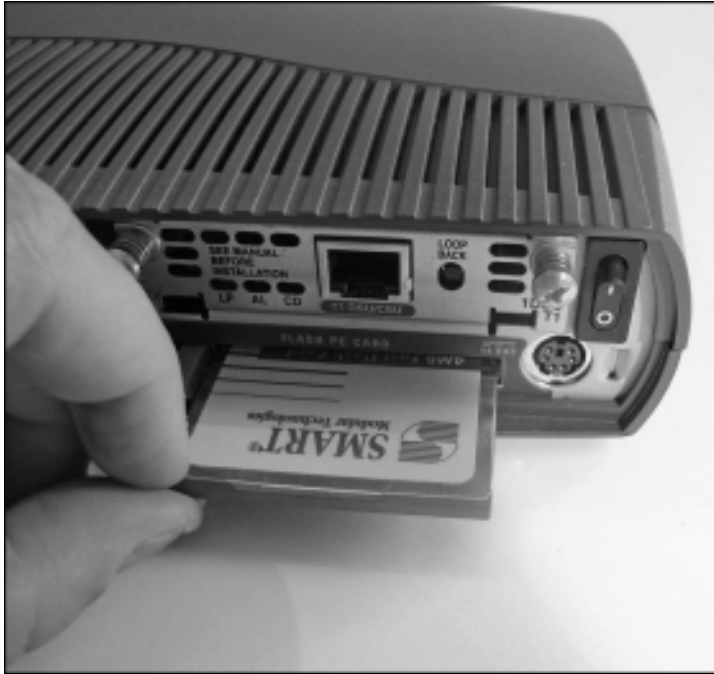
Figure 1-14: Installing a flash memory card on a Cisco router.
