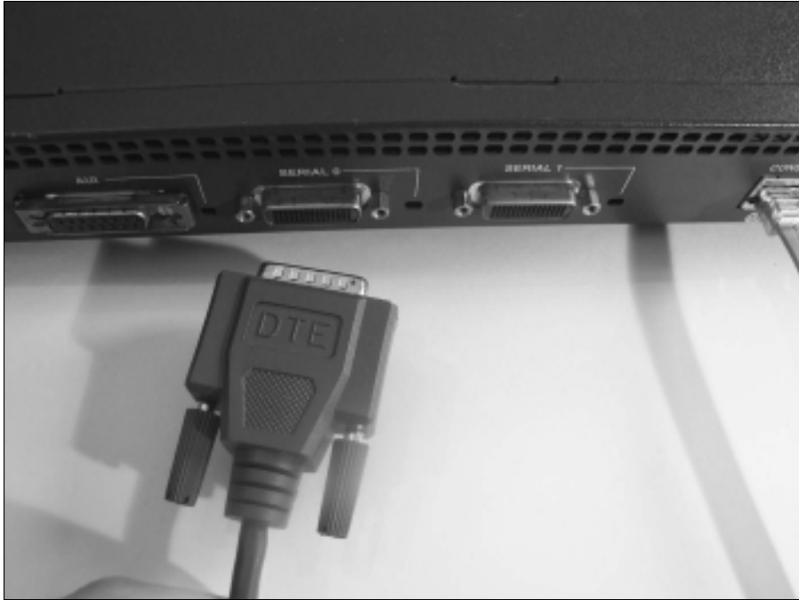
Figure 4-4: You can use a DTE/DCE cable to create a point-to-point link between your routers.
