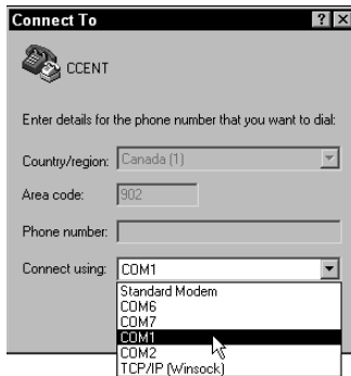
Figure 2-3: When connecting to a console port on a router from the serial port on your computer, choose COM1.
