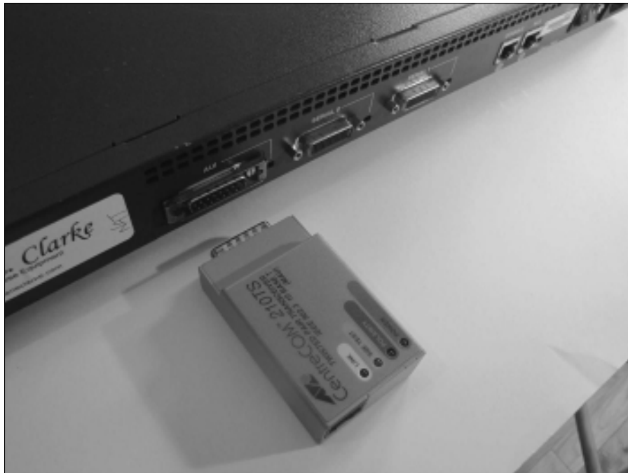
Figure 1-4: A transceiver connects to the AUI port on the Cisco router.
