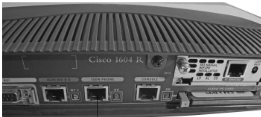
Figure 4-6: An ISDN port built in to the Cisco router is used to connect to an ISDN network.
