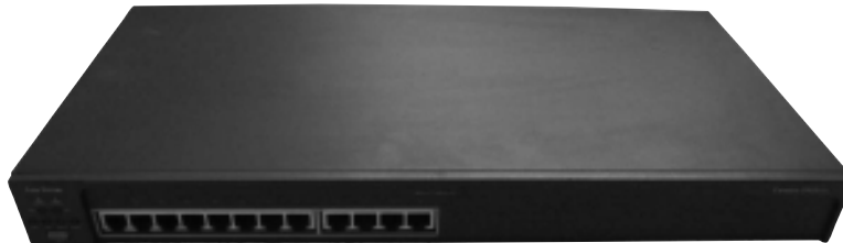
Figure 3-7: Each port on the switch acts as its own network segment.
