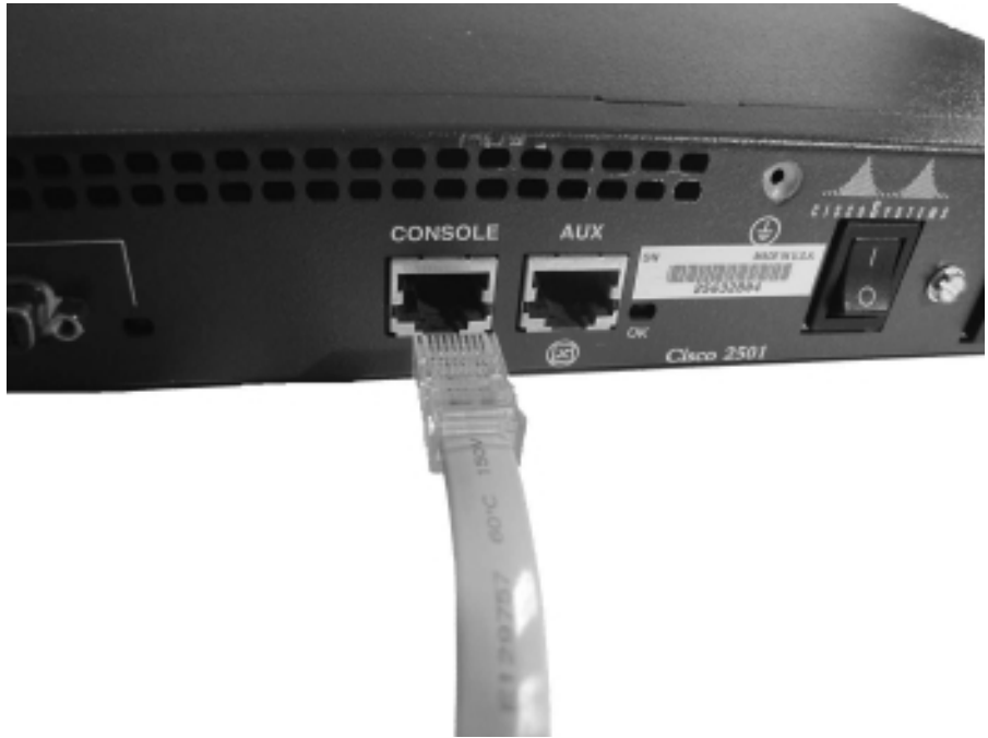
Figure 1-2: Connecting a workstation to the console port to perform local administration.
