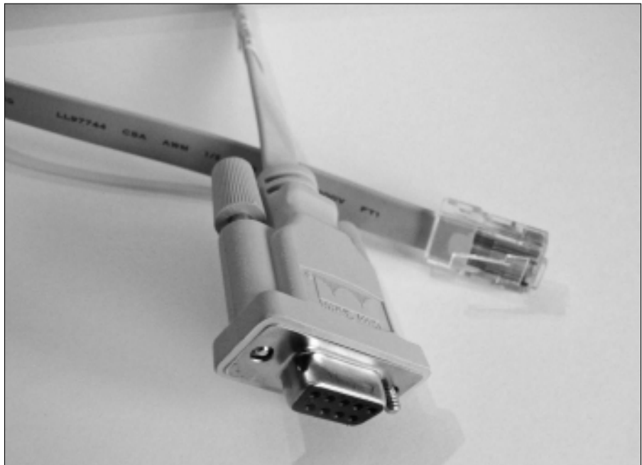
Figure 2-15: A rollover cable is used to connect your system to the router or switch in order to configure the device.
